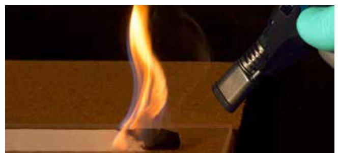
Test Apparatus: Powder 250 mm long train flame transiting length of the sample. The Fire Train mould prepares sample pile in a V-line for the burning rate test
