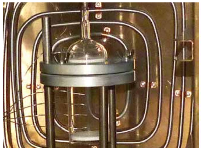
Aerated cell with pre-heated air (top entry)
