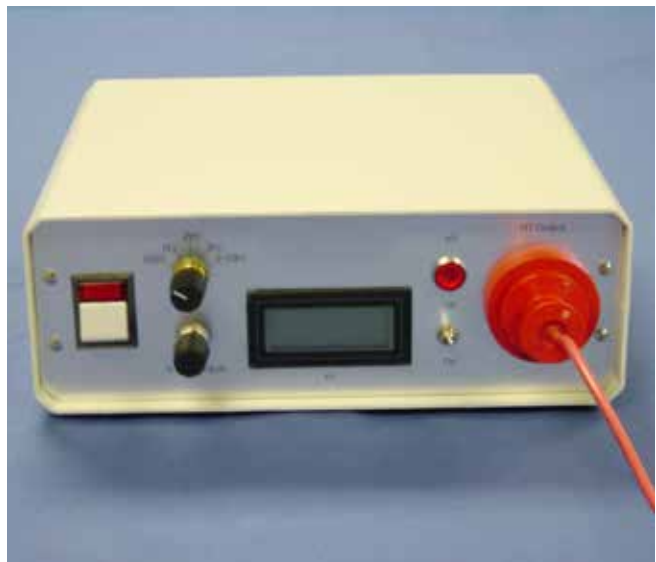
DEKRA Process Safety 10 kV Power Supply
